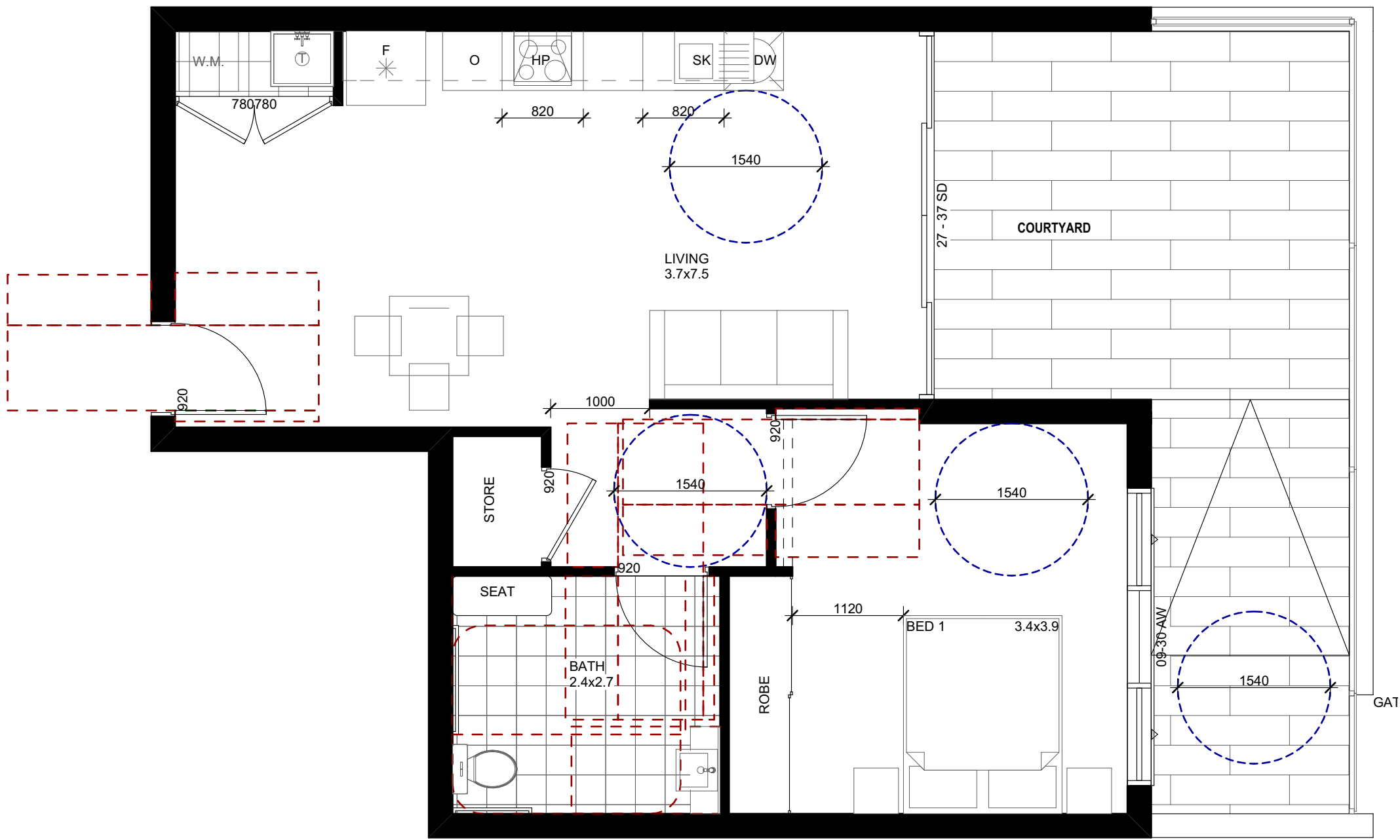
POST ADAPTATION PLAN - UNIT G.10 Scale 1:50
